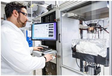
Various methods are used at Fraunhofer LBF to characterize the recyclates and compounds, for example flame retardancy tests in accordance with UL 94 for test specimens. Photo: Fraunhofer LBF, Raapke
