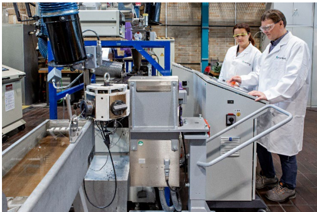
Online rheology at Fraunhofer LBF supports compound developers and makes formulations more cost-effective. Photo: Fraunhofer LBF, Raapke
