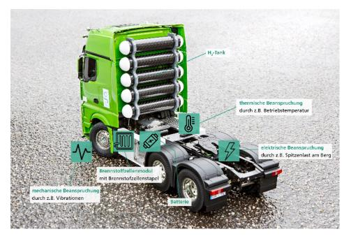
In "multiPEM", Fraunhofer researchers are evaluating the system reliability of fuel cell stacks under multi-physical-chemical stress in commercial vehicles. Graphic: Fraunhofer LBF
