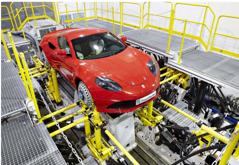
Fraunhofer Frecco 2.0 concept vehicle on the full-vehicle test facility in Darmstadt. Photograph: Fraunhofer LBF.
