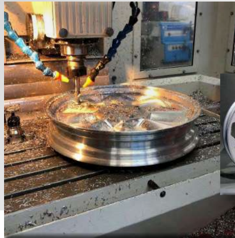
Entwicklung leichter Räder, z. B. für Cargo-Bikes. Development of lightweight rims, e.g. for cargo bikes.
