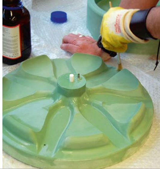
Bearbeitung der Radformen bei der Fertigung. Work on the wheel shapes during the manufacturing process.
