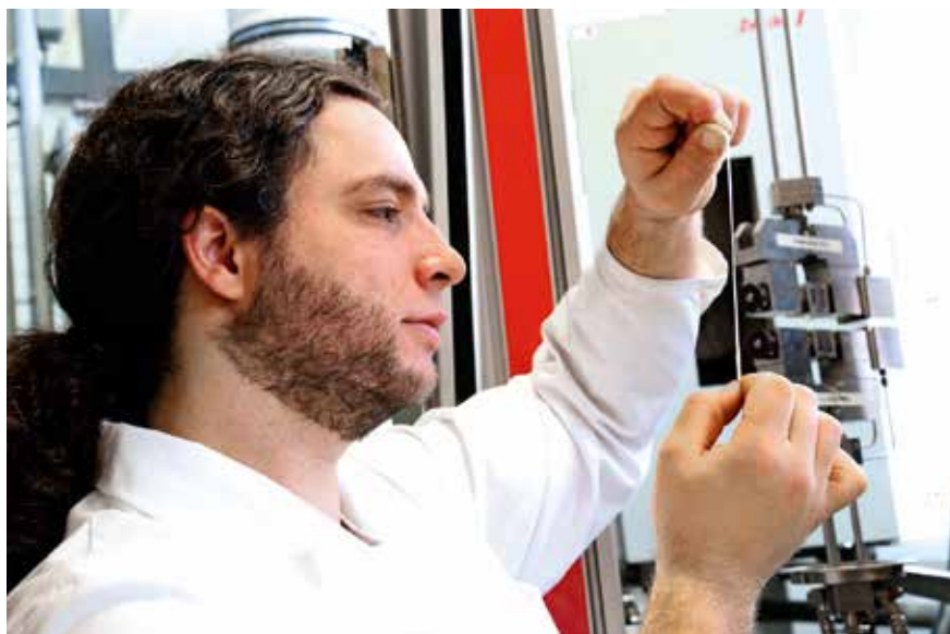
The reduction in tension set provided evidence of the partial crosslinking of TPS (figures: LBF)
